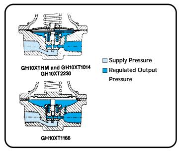
Figure 2. GH10 Series. No Bleed/No Relief Diaphragm
