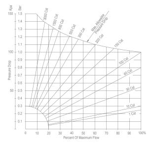
Model 85025: 100% = 160 l/min Model 85040: 100% = 250 l/min
