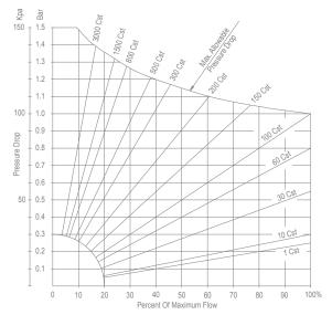
Model J5025E: 100% = 160 l/minModel J5040E: 100% = 250 l/min
