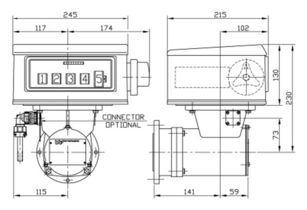
Fig. 3 Resetable flowmeter register
