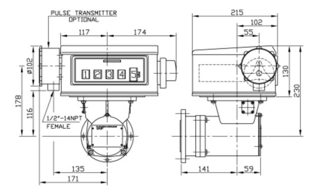
Fig. 4 Resetable flowmeter register with external pulse transmitter
